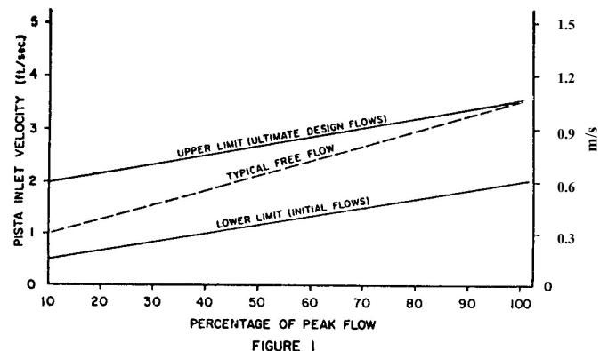
2 fps (0.6 m/s) is required to wash any grit that may have accumulated in the inlet flume at the lower flows into the grit chamber for removal.
